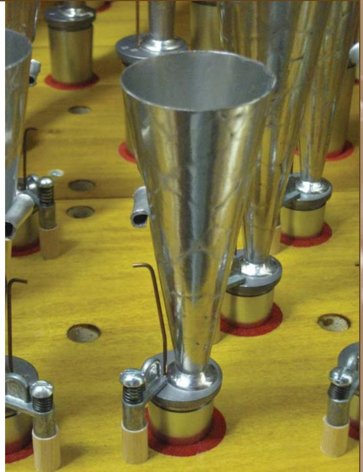
*Above is a pipe of the new Festival Trumpet. The wind pressure that blows into this reed is so high that the pipes needs to be fastened in place, or they will be pushed out of position.*
