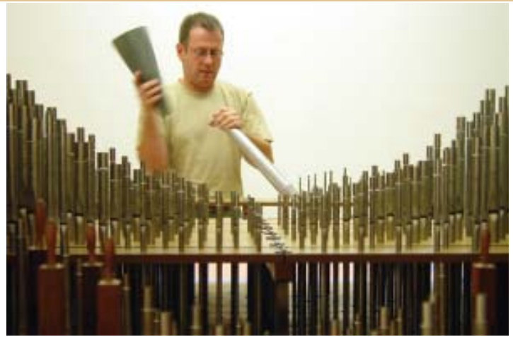
Jim Bennett, member of the Foley-Baker crew, adjusts the tuning sleeve on a pipe in the choir division.
